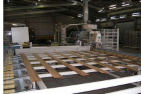
transfer table at end of spray line
